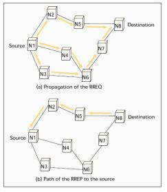
equal to the sequence number of the RREQ. Since the RREQ propagates by nodes passing it forward to its neighbours, an intermediate node will receive the same RREQ from many neighbours. Only the first copy of the RREQ is treated all others are discarded.
