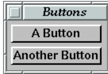
Figure 17. The same GUI elements as in Figure 15, but the program explicitly specifies vertical layout.
