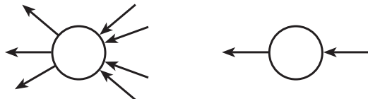
Figure 26. A general stream processor and a stream processor with a single input stream and a single output stream.
