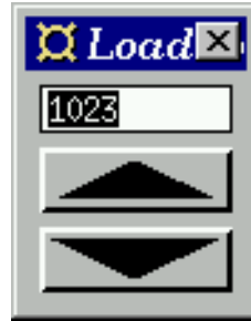
Figure 7. The loadable up/down counter.
